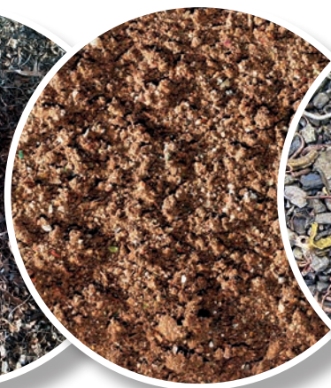
Output material Shredder Sand, free of metals
