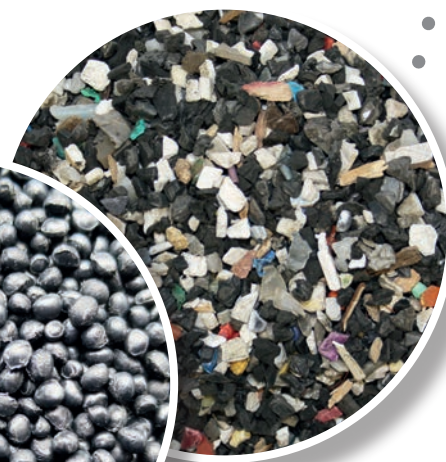
Output material ABS / PS / Filled PP (further separation possible)
