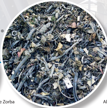
Input material (A)SR Shredder Residue
