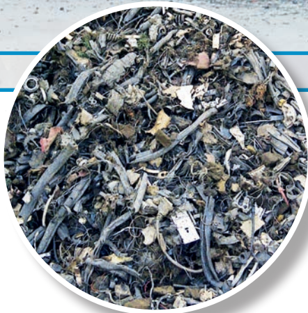
Input material (A)SR Shredder Residue
