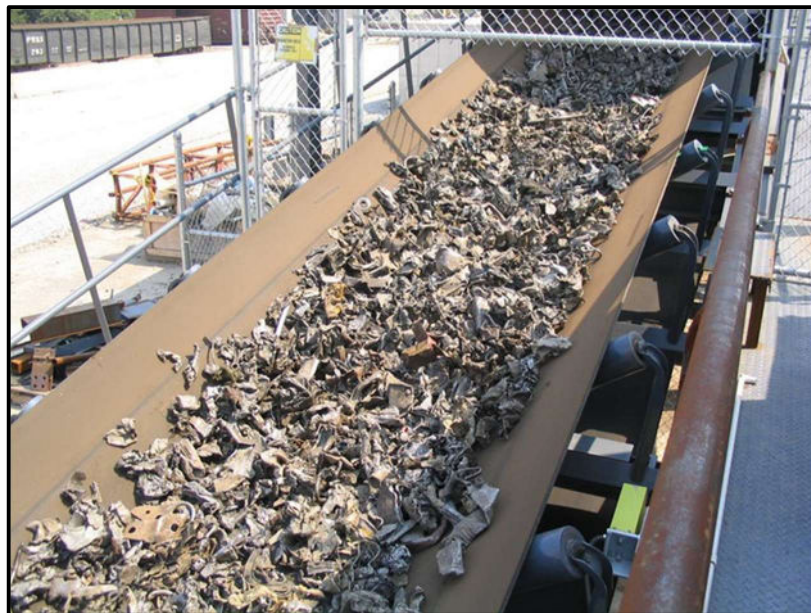
Figure 11: cross belt recycled metal analyzer (CB-RM)
