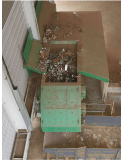
Figure 8: EcoRip®Neo for HMS Preprocessing
