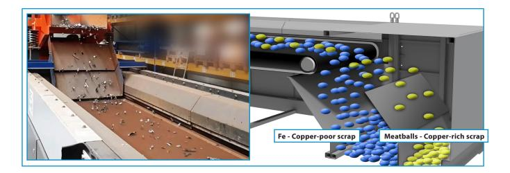
SICON's PrimeScrap is used for efficient cleaning of shredded scrap to have meatballs, non-ferrous materials or non-metal materials removed from the main material stream.
