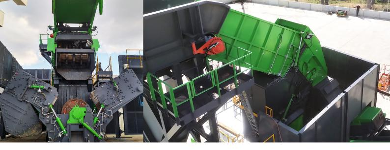
The EcoShred® Compact process results in a high and consistent scrap density and thus a correspondingly good material preparation – with clear advantages for the recovery of non-ferrous metals. The EcoShred® Compact forms the basis for the efficient operation of a shredder system.
