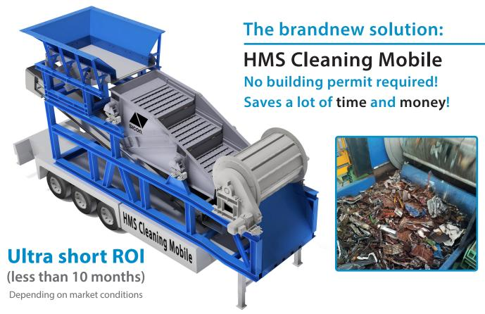
Improving the quality of steel scrap is for SICON the driving force behind the Heavy Metal Scrap (HMS) preparation process. HMS is cleaned intensively and NF metals that are still present are separated. The result is a scrap quality with a considerably higher Fe content and reduced NF content (specifically copper and aluminum).
